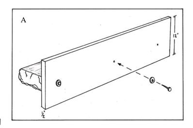
Next, take the mantel and plywood assembly and lag through the plywood into the wall studs at the location you desire as shown in **Figure B** at right.
